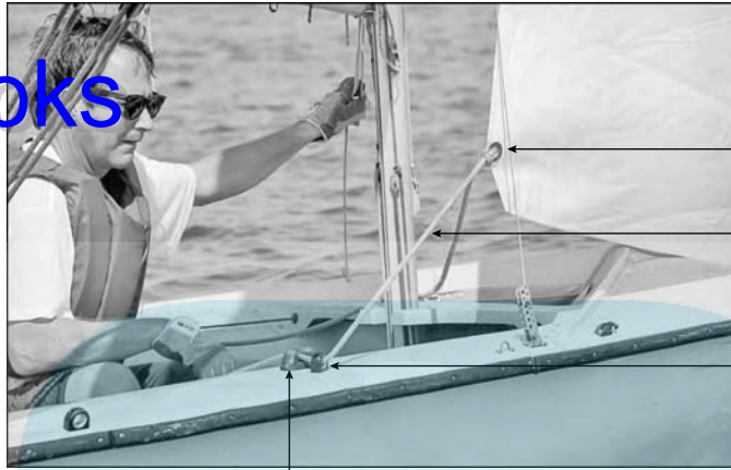
Figure 4-11: Jib sheet system on a 420-class dinghy.
